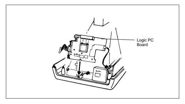
Figure 5-10 Logic PC Board
